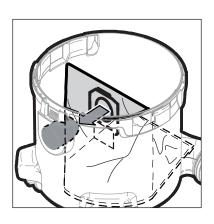
4. Press the filter bag connection firmly on to the inlet fitting.
