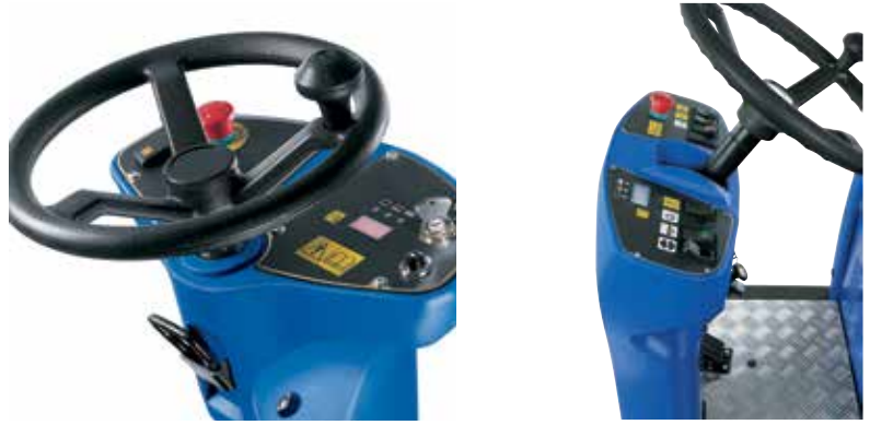
The steering column adjusts to fit the operator and to ensure easy access to the machine.
